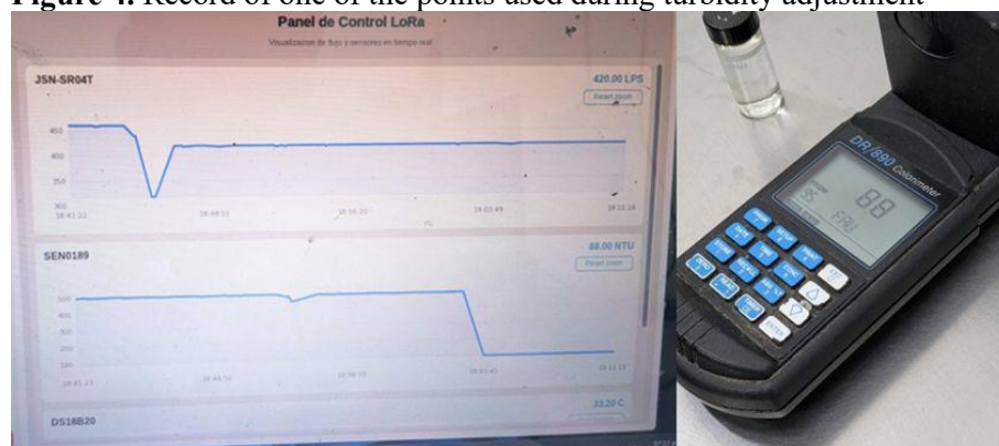
Figure 4. Record of one of the points used during turbidity adjustment
